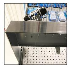
2) Confirm all the shelves are at the correct height. If not adjust the shelves to the notches as shown below:
